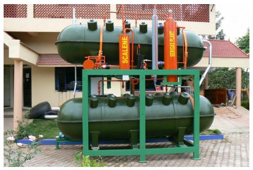
SERI has developed a highly-controlled biological reaction process comprising the use of specifically cultured microbial ecosystem for aerobic and anaerobic digestion of organic feedstock, including food waste, non-consumable part of fruits, vegetables and other agricultural waste, municipal solid waste, oil effluents, animal, poultry and fish waste, excreta of humans and animals, and weeds such as water hya-
